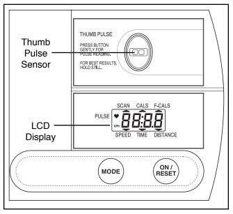
Speed—This mode displays your pedaling speed, in miles per hour.
